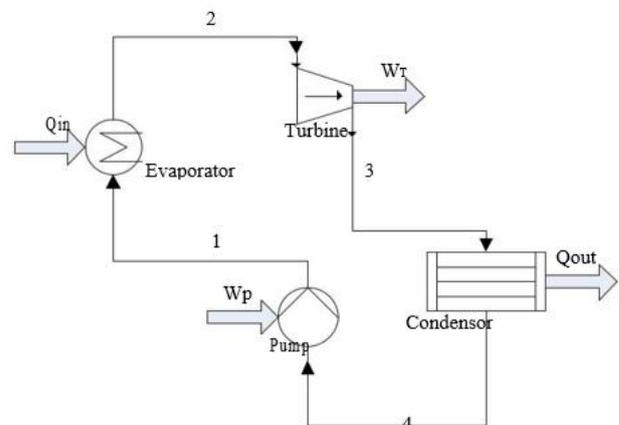
Fig. 2. Simple Cycle of Organic Rankine Cycle
