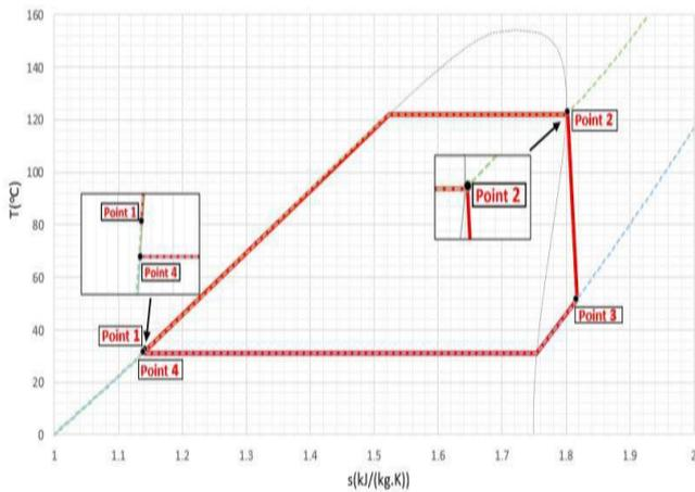
Fig. 3. *T-s* curve of the system
